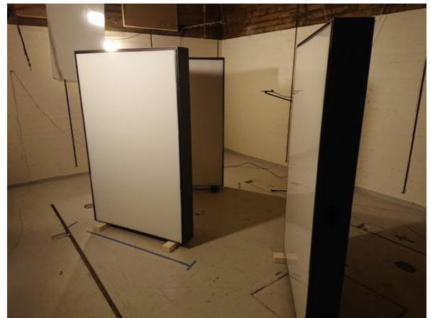
Figure 4: Three Lintex Unit 1800x1200 mm glass/glass, measured for sound absorption.
